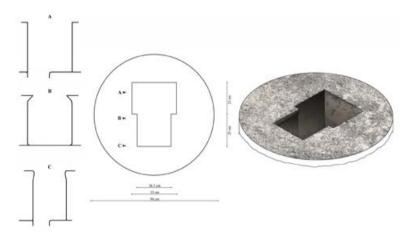
Fig. 5.34 The SW screw mortice, a plan and sections.
