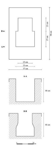
Fig. 5.30 The NE screw mortice, a plan and sections.
