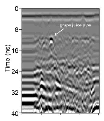
**Fig. 5.36** Ground-penetrating radar results at the SE treading floor. Small reflection hyperbola caused by a pipe for grape juice to flow into a vat.
