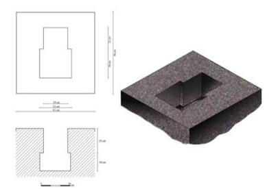
Fig. 5.32 The SE screw mortice, a plan and sections.
